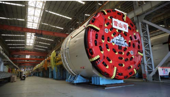
中交天和研发生产的“雪山号”盾构机用于天山胜利隧道施工 The "Xueshan" shield tunneling machine researched and developed by Tianhe is applied in the Construction of Tianshan Shengli Tunnel
